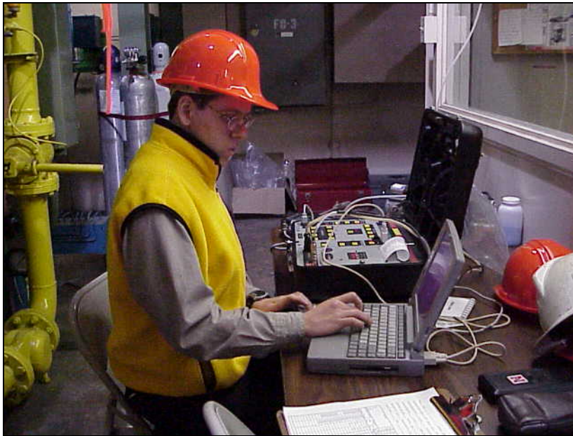
Fig. 14. Logging of emissions data from Enerac 3000E.
